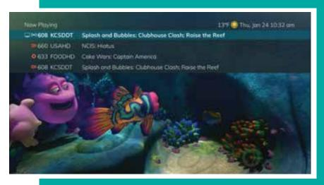
In this example, the TV symbol indicates you are viewing Splash and Bubbles from channel 608. The antenna symbol next to channel 608 indicates that it is on live television. Channel 660 is currently recording as part of a series recording indicated by the red circle with lines next to it. Channel 633 is currently recording as indicated by the red circle. Channel 608 is also recording as part of a series recording indicated by the red circle with lines next to it.
